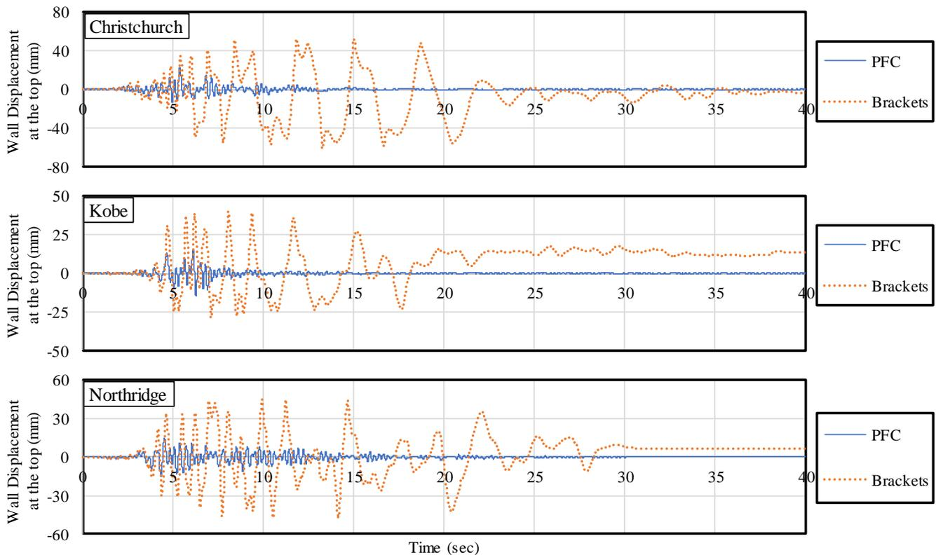
Figure 9. A comparison of displacement time-histories. Top: Christchurch; Middle: Kobe; Bottom: Northridge.
