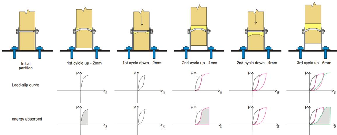
Figure 2. Pinching phenomenon observed in traditional bracket hold-down connectors.
