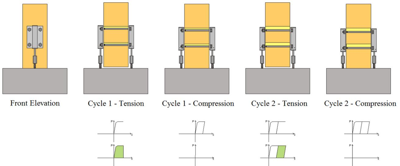
Figure 3. Slack is eliminated on each cycle by the proposed connector, providing a hold-down connection free from pinching.
