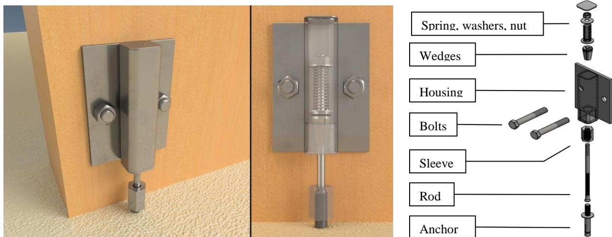
Figure 4. The pinching-free concept applied as a hold-down for rocking shear walls.
