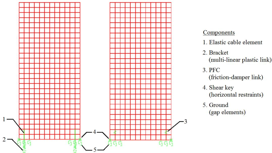
Figure 8. Shear wall models equipped with ordinary bracket connections (left) and pinching-free connections (right).
