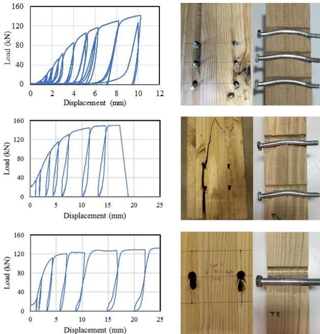
Figure 7. Hysteresis and specimen of the three connections tested. Note that the x-axis scales are adjusted for clarity.
